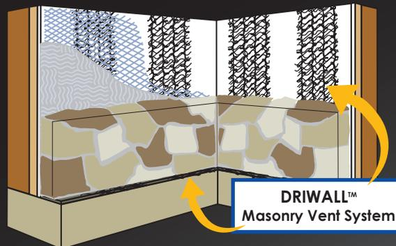
**DRIWALL Masonry Vent Strips** are the most economical solution for draining and ventilating masonry walls. The product creates a vertical ventilation strip approximately every two feet along the wall. That strip is allowed to exit the wall at the bottom creating the path for liquid moisture to drain and for air to circulate.
