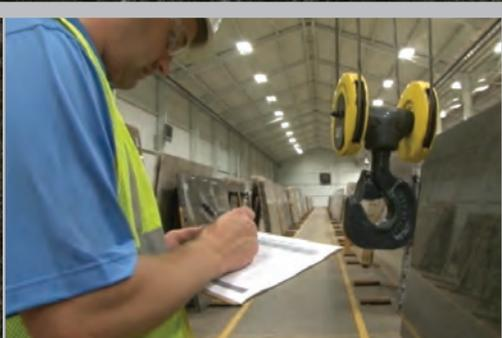
Worker with inspection checklist for hoist
