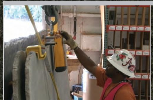
*Clamp being properly positioned*
