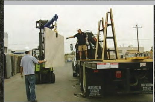
*Loading a slab onto a flatbed truck with an A-frame*
