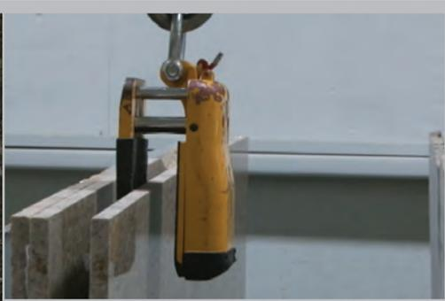
*Positioning clamp for safe lifting*
