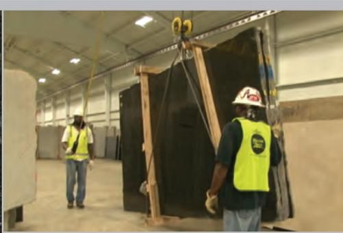
*Moving a slab with an overhead crane*
