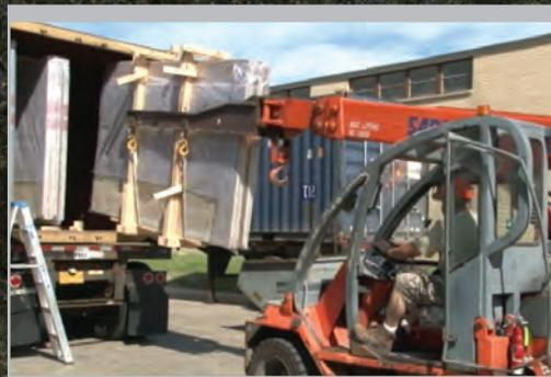
*Mobile crane extracting a bundle from a container in an outside stone yard*
