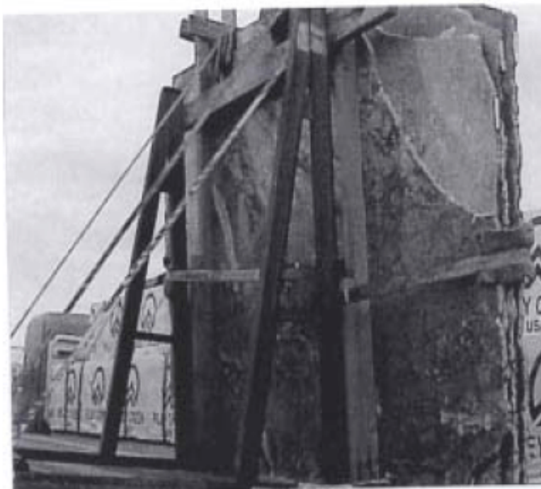
Close-up of A-frame rack used to transport rock slabs
