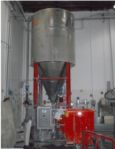
Silo where flocculation and particle separation occur. The red apparatus to the right is the filter press.
